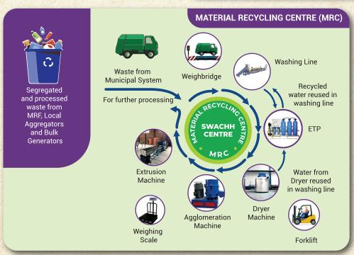
MRCs have washing lines, dryers and effluent treatment plant (ETP). This is supplemented with extrusion machines to make different types of granules.
